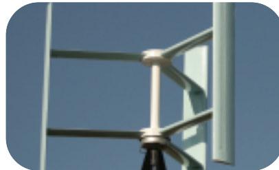
Vertical Access Wind Turbine
